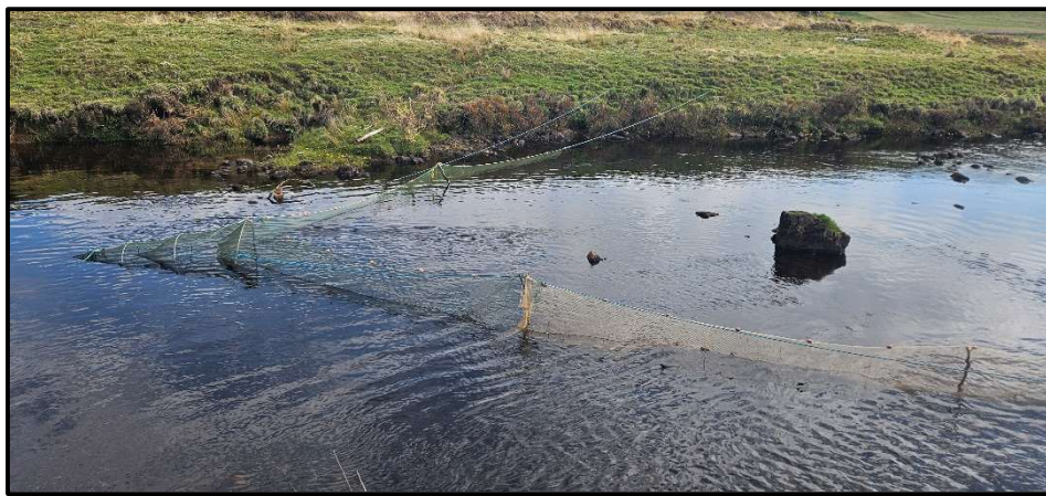
Figure 4. Estuarine fyke net deployed in the River Snizort during the spring 2024 salmonid migration.
